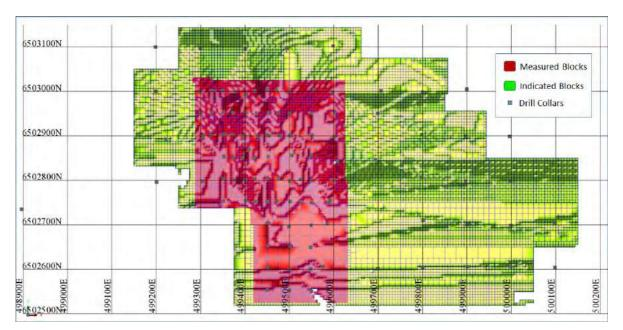
Figure 14.12Resource Classification of Blocks – Plan View
