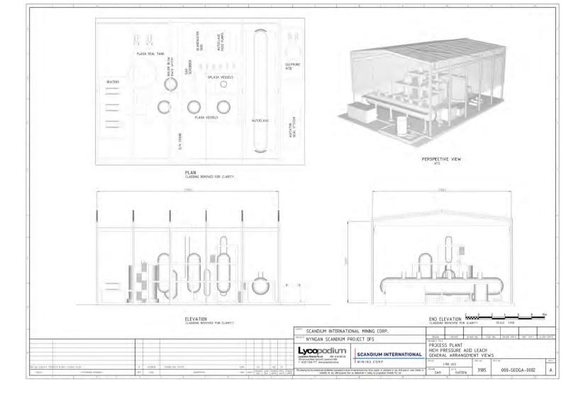
Figure 17.3 High Pressure Acid Leach Area Layout
