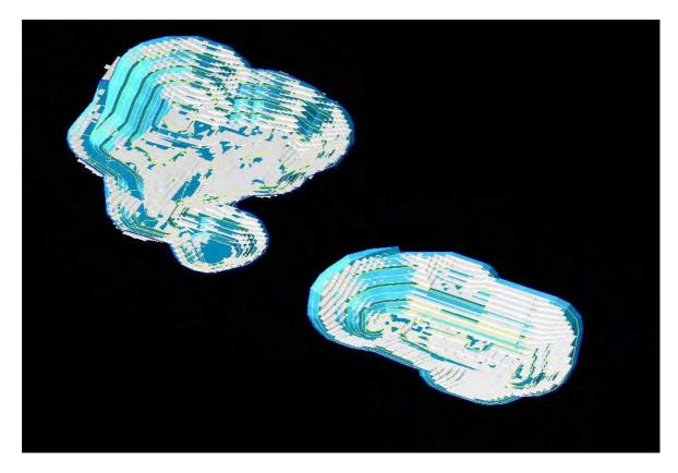
Figure 16.7 Whittle Shell against the Pit Designs
