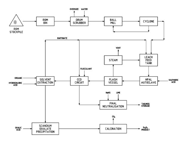
The solvent extraction and precipitation programs conducted in 2015 have resulted in an evolution of the flowsheet compared to that developed by other researchers in the following areas:
