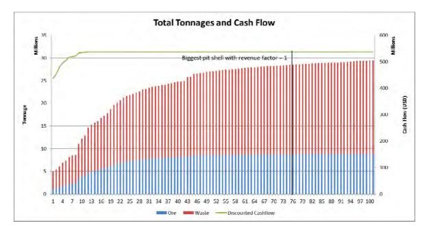
Figure 16.2 Whittle Optimisation Results – Optimum Shell 76
