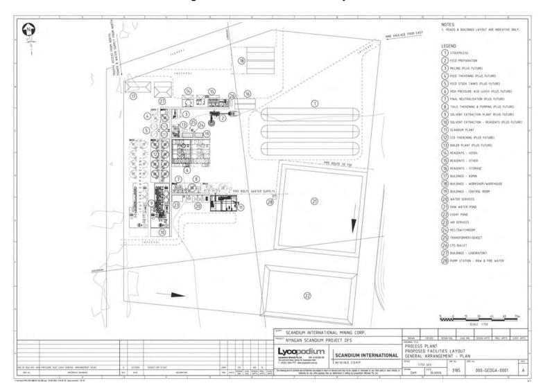
Figure 17.2 Process Plant Layout
