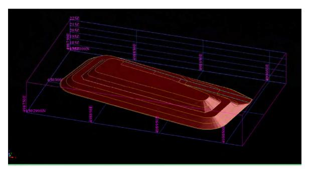
Figure 16.21 Low Grade Stockpile Design Profile
