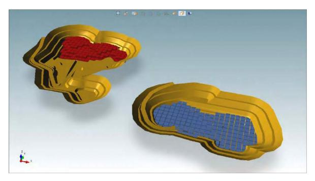
Figure 16.13 Mine Pit Configuration – Year 10
